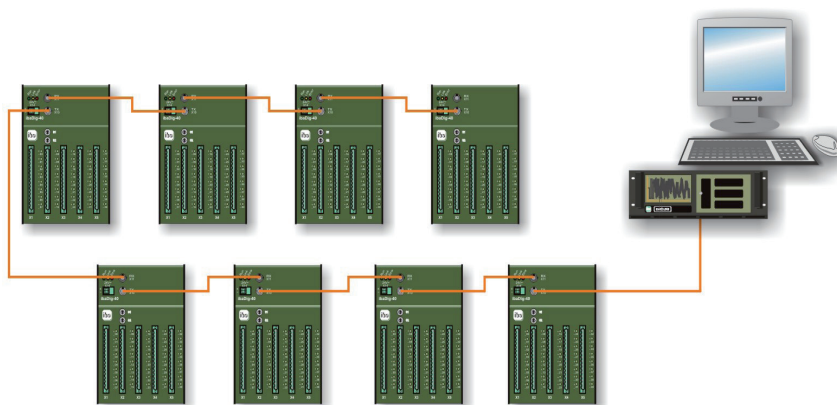
Daisy-chain topology with 8 ibaDig-40 devices along one fiber optic line
